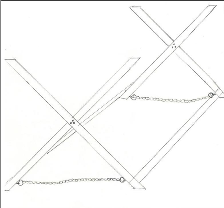
Mark built an X frame to hold the barrel. Keep in mind, a barrel full of compost will be quite heavy! The frame supporting the barrel needs to be quite strong and stable.
